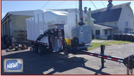
ated by a wireless remote control from the cab of the truck. The wireless camera system will aid the driver in maneuvering the suction arm during operation. The automated arm system reduces the need from 3 employees down to 1.
